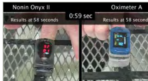
Figure 3: Nonin Onyx keeps reading while passing the 10 minute IPX2 moisture exposure test. Oximeter A stopped reading at 58 seconds. 7
